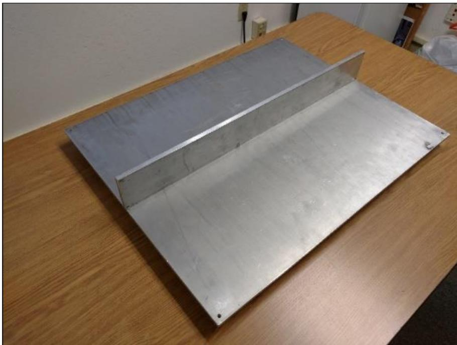
*Plate with RIB Stiffener Attached*
