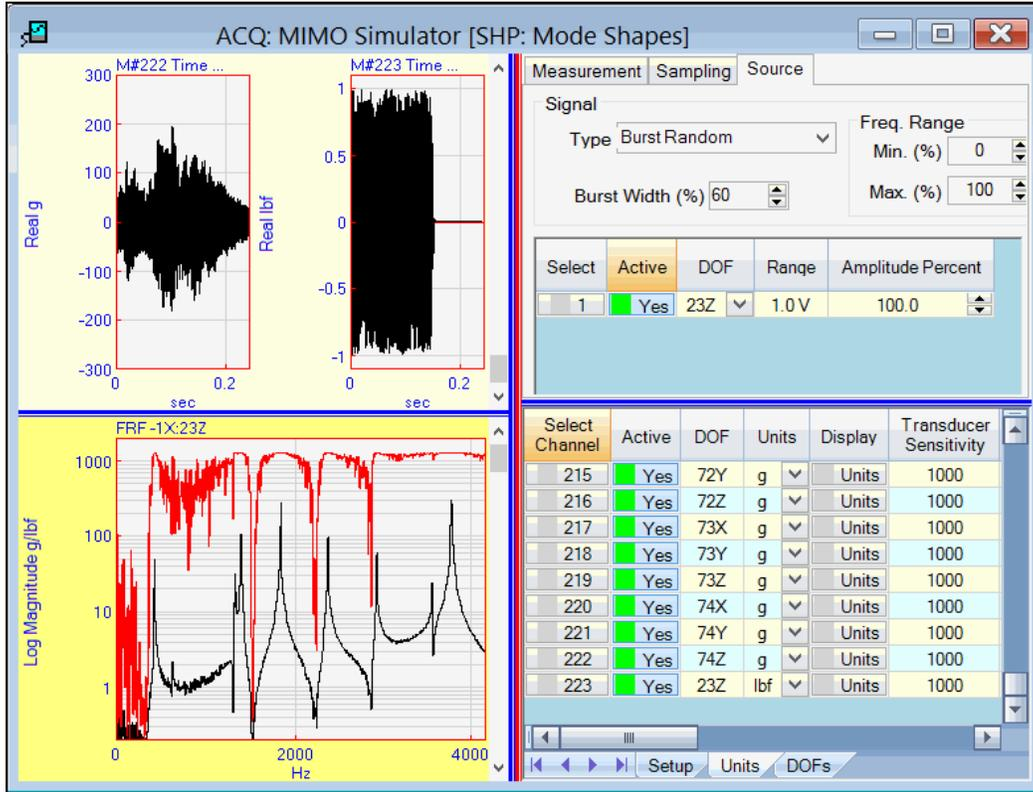
Source Tab Showing Burst Random Output from Source Channel 1.
