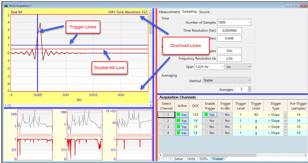
Acquisition (ACQ) window After Triggered Acquisition Has Occurred.
