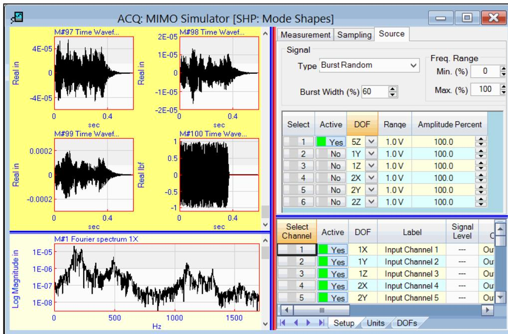
*Correct Burst Random Output Showing Responses Contained in The Window.*
