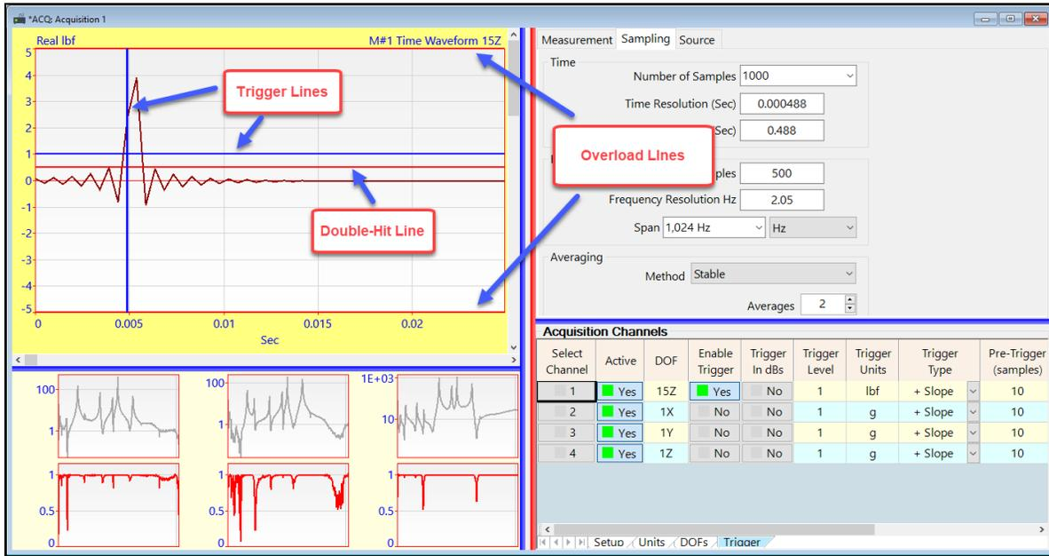
*Trigger, Double-Hit and Overload Lines on the Upper Graphics.*
