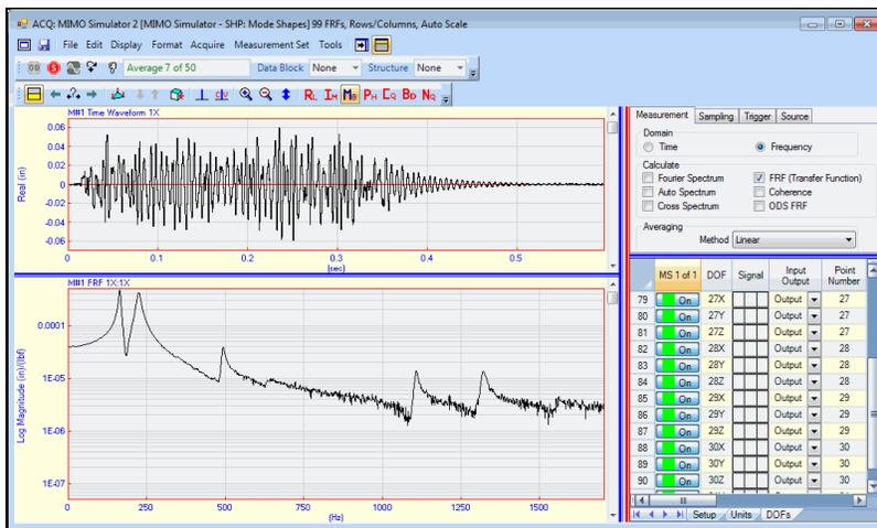
Acquisition (ACQ) window during Data Acquisition.
