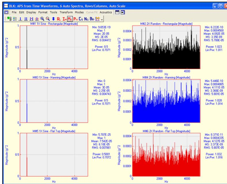
*Narrow Band and Wide Band Spectra Power Corrected for Windowing.*
