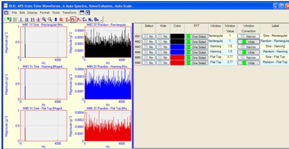
*Narrow Band and Wide Band Spectra Amplitude Corrected for Windowing.*
