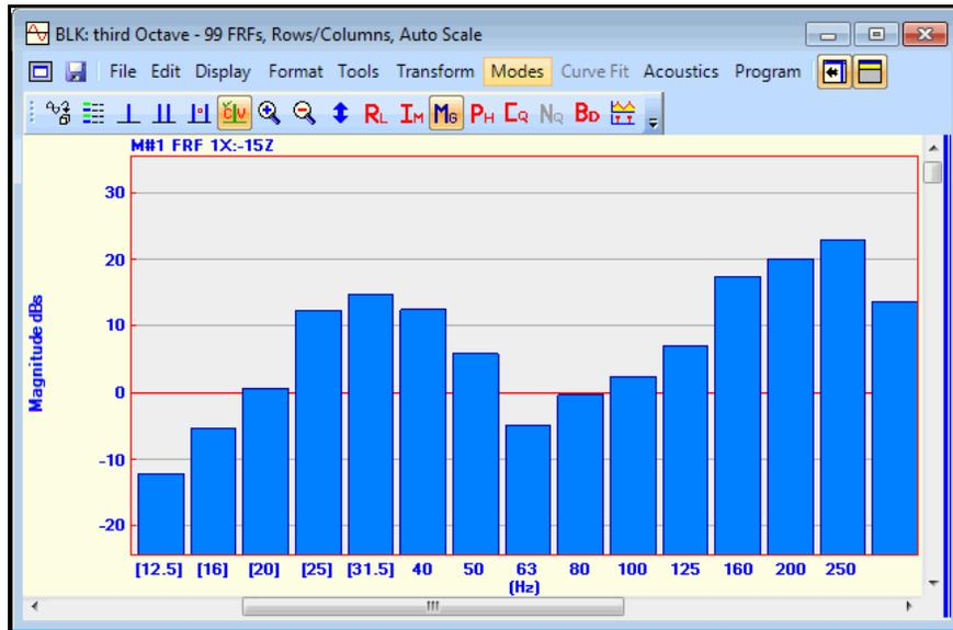
*Octave Band Measurement Showing Bands Created from Less Than 5 Samples.*
