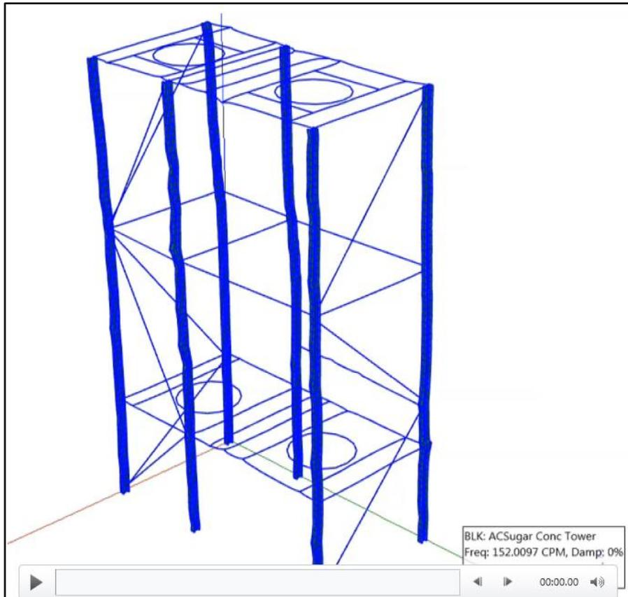
Figure 7. ODS of the Tower from Accelerometers
