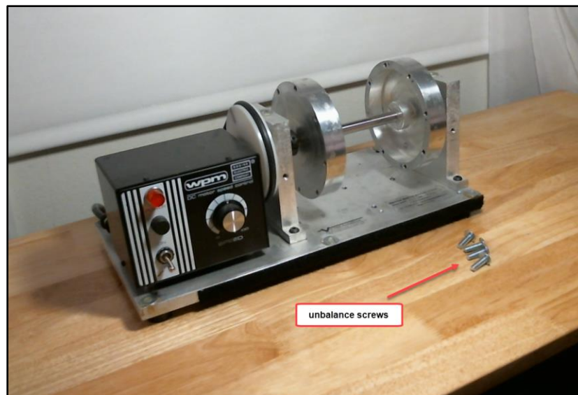
Figure 1. Rotating Machine Showing Unbalance Screws Added to Its Rotors
