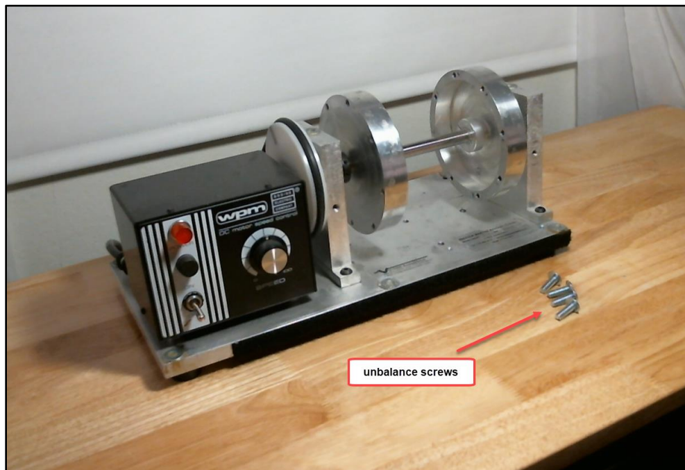
Figure 1. Rotating Machine & Unbalance Screws Added to Its Rotors
