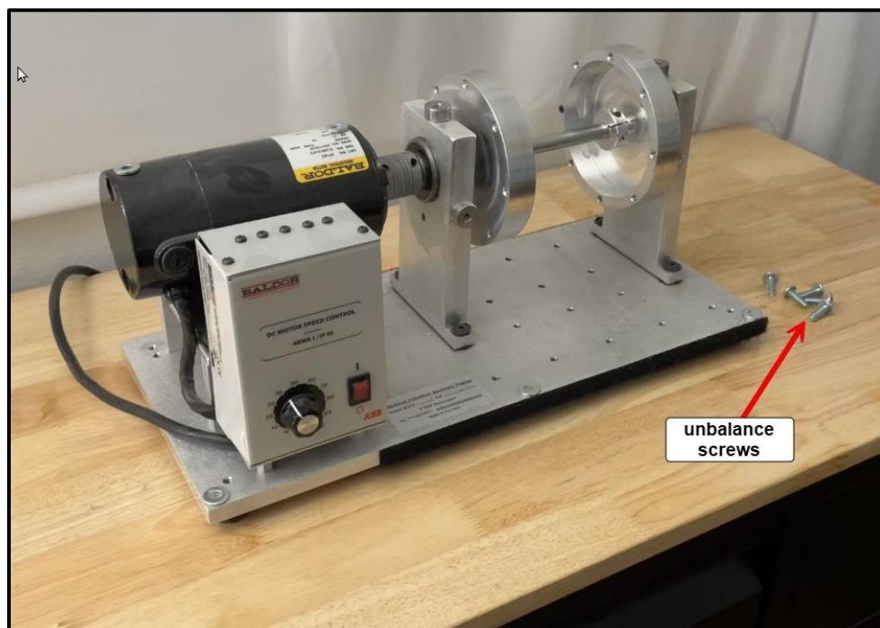
Figure 1. Rotating Machine With Unbalance Screws Added to Its Rotors
